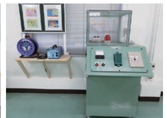
Electrical leak simulation device
