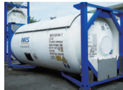
HFO-1233zd(E) ISO tank container (Reprinted with the permission of the NRS Corporation)
